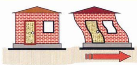
Effect of Inertia in a building when shaken at its base
